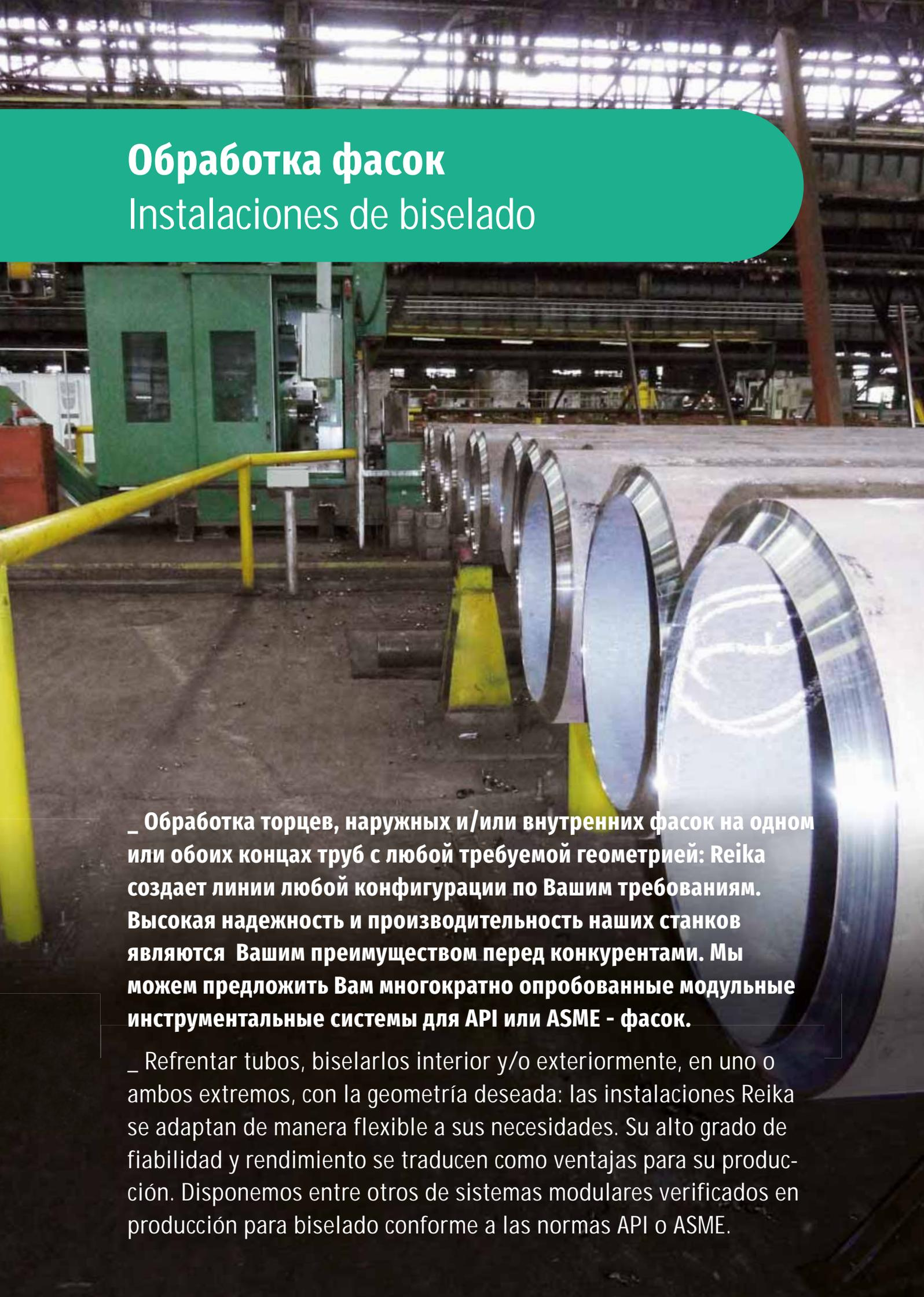
A photograph of a large industrial facility, likely a steel mill or pipe manufacturing plant. In the foreground, a row of large, dark-colored metal pipes is lined up, each with a beveled end. The pipes are supported by yellow chocks. In the background, there is a large green industrial machine with a yellow railing in front of it. The ceiling is high with a complex network of steel beams and lights.
